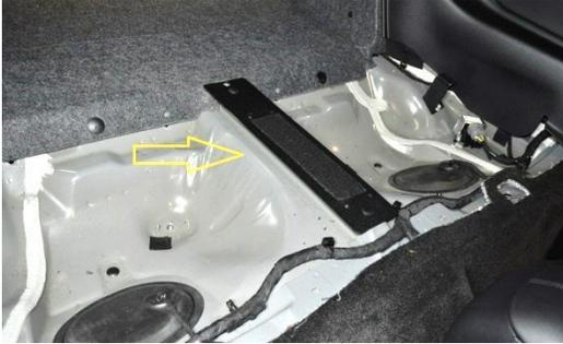
1. ← Install the flat center brace over the transmission tunnel using the two fat plastic push pins included in the hardware kit. One push pin goes in the **threaded hole** near the back. The other pin **with tape**, goes in the front hole. The tape is there to make a tighter fit. You can add or remove tape to get the desired fit.
