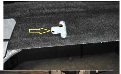
15. Reinstall the left and right factory side panels back in the car. Push firmly on the panel to seat the clips.
