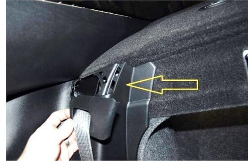
5. ← Remove the rear side panels by firmly pulling away from the body of the car to release the plastic clips holding it in place. This may take more force than you think is comfortable, but just pull firmly around the edges and each one will release. Temporarily remove both of them from the car.
