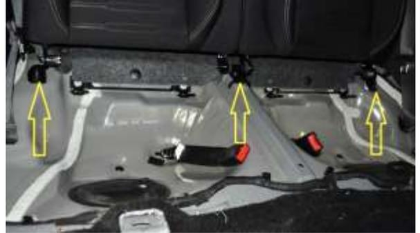
3. ← Fold the seat backs down. There is one more nut to remove at each side near the side panels. Remove the seat backs from the car.
