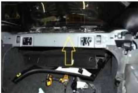
12. ← With the side panels gone, you can temporarily remove the factory carpeted rear deck panel. This will be reinstalled in a later step.
