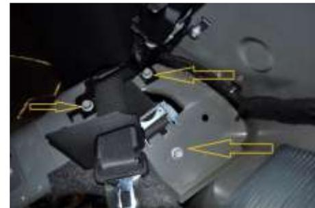
6. → You now have access to the 3 bolts holding the seatbelt mechanisms. Remove these 3 bolts on each side and pull the mechanism out of the hole. →
