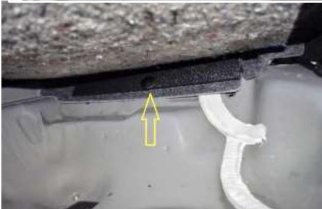
4. ← At the back of the lower panels there is a notch built-in to sit on top of a threaded stud that protrudes from the body of the car. There is a factory black plastic cover over this stud. The new lower panel should go **BEHIND** this plastic stud cover to help hold it in place.
