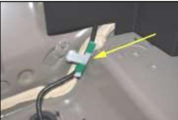
5. ← At the rear trunk wall, you will need to unhook the wiring harness holder from the metal tab, and tuck downwards. This prevents interference with the rear seat delete.
