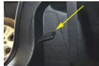
6. At the rear upper portion of the interior trim is a removable access panel on each side, where the seats previously connected to. To remove the black metal bar, carefully pry this access panel open, and remove the bolts holding it in place. Reinstall the access panel. →
