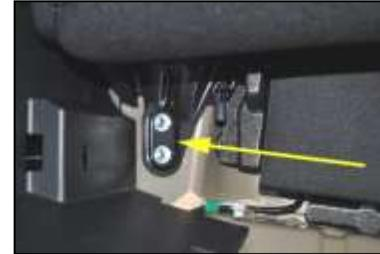
4. In the rear trunk area, remove the 4 mounting bolts for the assembly as shown. The entire seat assembly must be lifted out as one unit, so be careful not to scratch your interior panels! →
