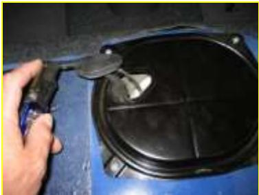
4. ← **(NOTE: 500C Cabrio skip this step)** Use a knife to carefully trim back the black tape that keeps the rubber grommet in place. Pull the wires about 3-4" out of the rubber grommet to give enough slack to move the wires to the other side of the hump. Make sure rubber grommet is still firmly in place to seal the hole.
