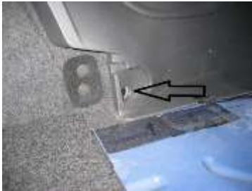
1. ← Install each of the supplied plastic side covers where your rear seat previously mounted at the side panels of the car. Use the factory black hex bolts you removed from this location earlier, to mount them.
