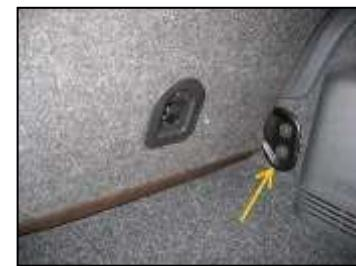
4. ← Remove the center seatbelt bracket. The 2 rear bolts are T50 Torx. The front hex bolt is a standard metric socket. Reinstall the hex bolt and Torx bolts, to plug the holes.
