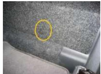
5. Mount the front edge of the rear seat delete panel using the 2 black factory Hex bolts you removed in an earlier step. It's hard to see in the photo but the circled area indicates the location. →
