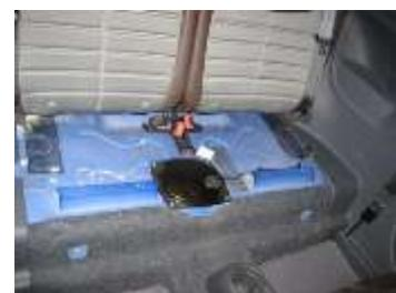
2. ← Lay seats down. Remove center hex bolt from the center bracket to release the 2 seat halves.
